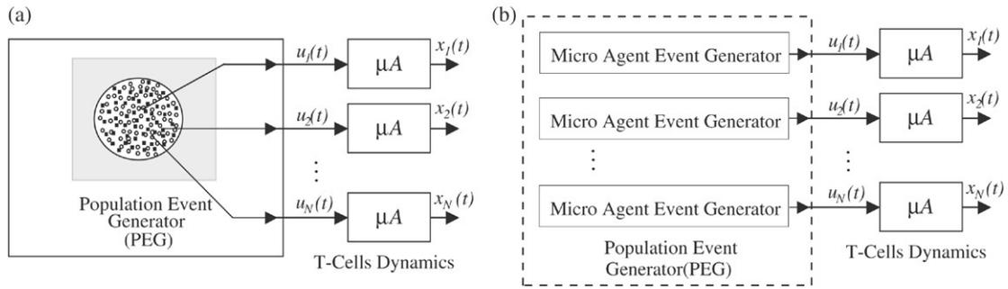
Fig. 4. The T-cell population model; (a) the hybrid system model  $u_i$  — event sequence input to the  $i$ th T-cell,  $x_i$  — the TCR expression of the  $i$ th T-cell,  $i = 1, 2, \dots, N$ ; (b) the population event generator (PEG) is decomposed into several micro-agent event generators (MAEG). The serial connection of MAEG and micro-agents is named a stochastic micro-agent,  $S\mu A$ .
